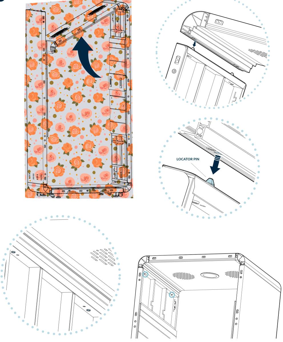
With one person holding the SIDE PANEL, have another person raise the CEILING PANEL and position the insert holes over the Locator Pins on top of the Side Panel. They will automatically position and secure the Ceiling Panel and loosely tighten using the included 6MM ALLEN KEY. Then insert (2) M8 X 45MM SCREWS into the insert holes located at the top of the Side Panel and loosely tighten using the 6MM Allen key.
