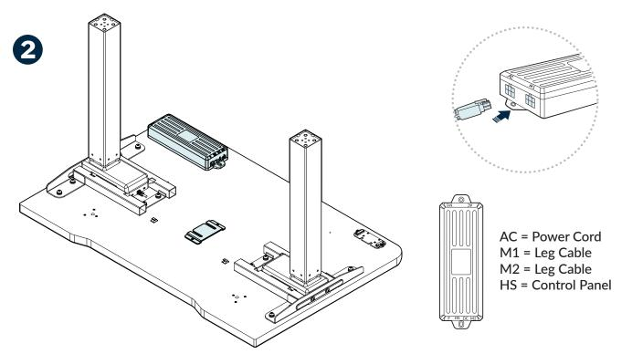
With the desk still face down and legs secured, lower the **CONTROL BOX** into the center cavity of the metal frame. Slide the control box to engage the bracket and lock it into place. Once secured, connect the **LEG CABLES** to the corresponding inputs labele **M1** and **M2**.
