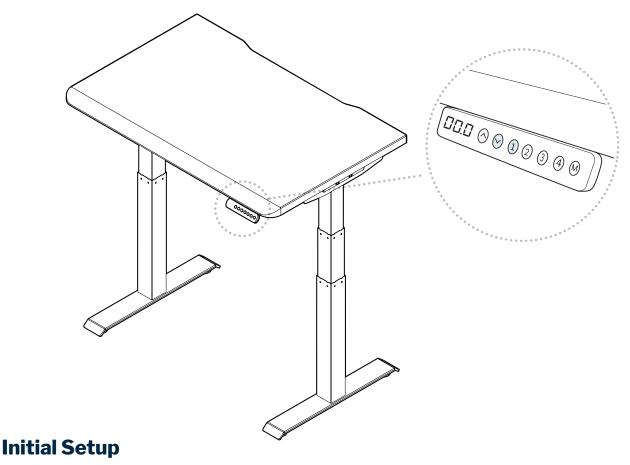
Press the DOWN button on the control panel until the base reaches its lowest position. Press and hold the DOWN button again until the LED display reads "RST".
