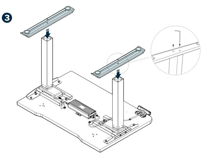
Once the control box is secure and while the desk is still face down, place one **FOOT** on top of one leg aligning the screw holes. Use the larger **HEX KEY (M10)** provided to securely tighten **(2) M10X40** screws into each foot.
