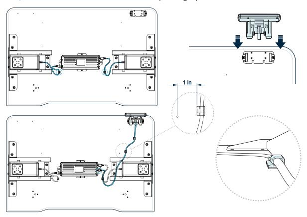
Locate the **CONTROL PANEL** and slide it into the bracket to attach. Once the panel is in place, connect its cable to the corresponding control box input, **HS**.
