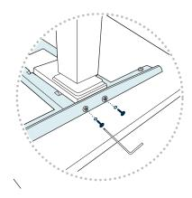
Use the smaller **HEX KEY (M6)** provided to securely tighten (2) **M6X14 SCREWS** and (2) **M6X14 WASHERS** onto each leg.
