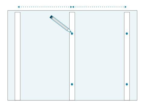
Use a stud finder to locate (2) ADJACENT WALL STUDS. Mark the center of each stud.
