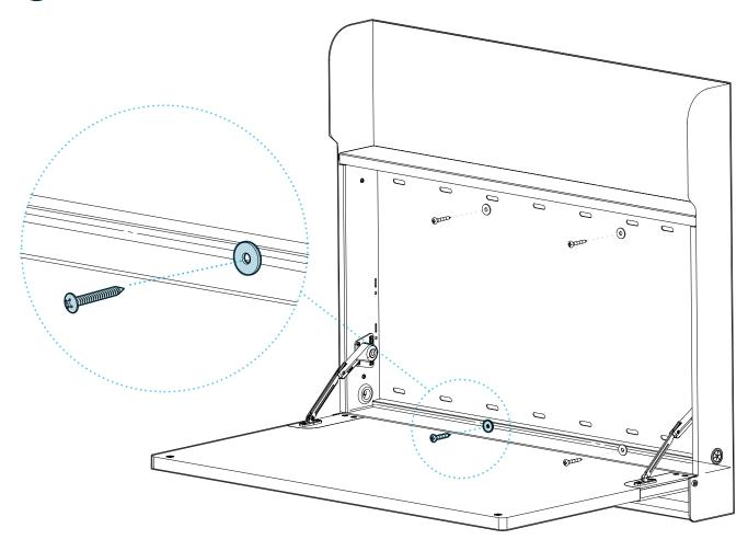
With another person supporting the desk, align it with the wall marks from the previous steps. Secure it to the wall studs by driving the (4) #10 X 1-1/2" SELF-TAPPING SCREWS and WASHERS through the back panel of the desk. Tighten the screws using a Phillips Head Screwdriver (not included) or Drill with a Phillips Head Drill Bit.
