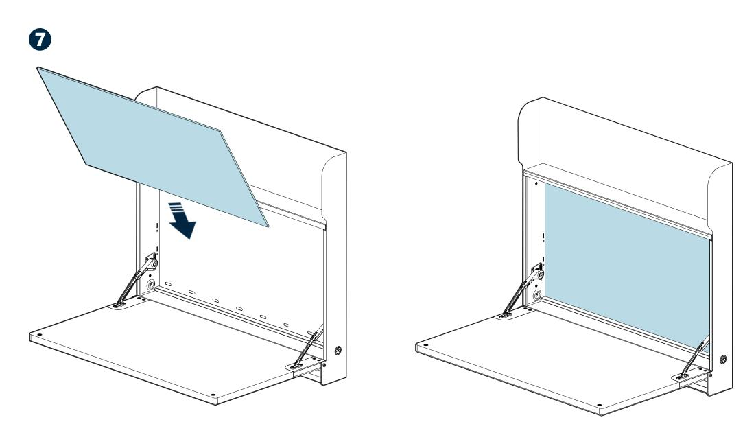
Insert the **PET FELT BACKING** into the desk and secure it to the back panel.
