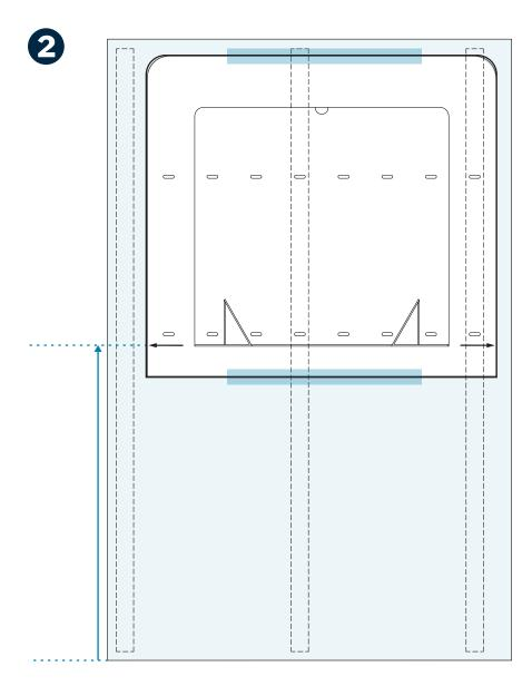
Place the **MOUNTING TEMPLATE** on the wall. aligning its holes with the stud marks from Step 1. Have another person hold it in position or secure it with painter's tape.
