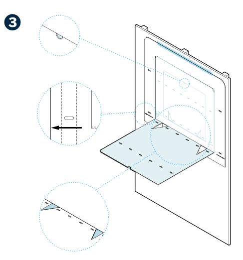
Pull down the mock worksurface and fold out the two triangle supports to keep it flat. For seated height, pull up a chair; for standing height, stand where you plan to use the desk.
