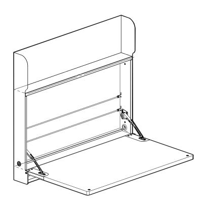
**WARNING:** Do not exceed a max load of 100 lbs on the worksurface; exceeding this may cause injury or damage.
