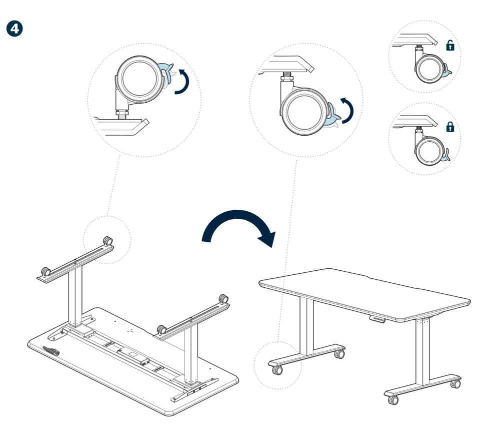
Insert the threaded post of each caster into the now-open holes. Use the provided 14mm wrench on the caster's nut to turn the caster clockwise until fully tightened.
