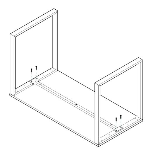
Secure the Legs to the Support Beam using four (4) M6-35 screws.
