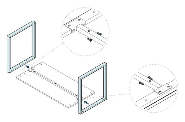
Secure legs to Support Bar with four (4) M6-20 screws. Hand-tighten only (do not tighten them completely).
