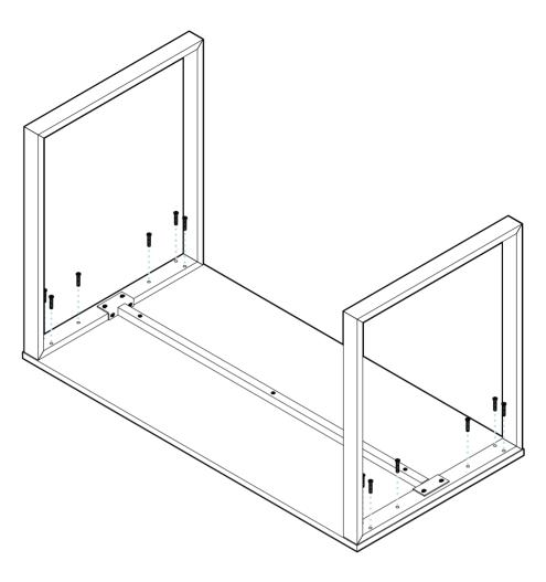
Using twelve (12) of the M6-30 Screws, secure the Legs to the Desk Top. **Using the Allen key, tighten all of the screws.**
