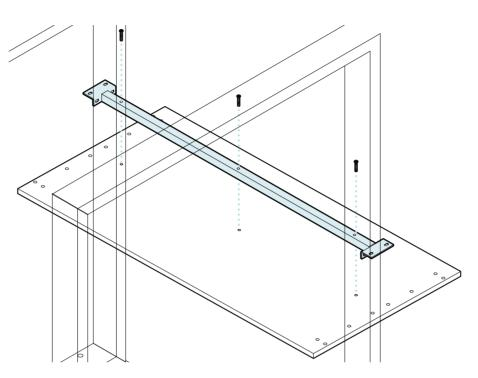
Place the Desk Top upside down on the box. Secure the Support Bar to the Desk Top with three (3) M6-35 screws. **Hand-tighten only (do not tighten them completely).**
