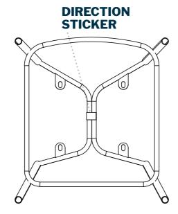
Position the seat with the front edge of the seat in the direction indicated on the sticker underneath the frame.
