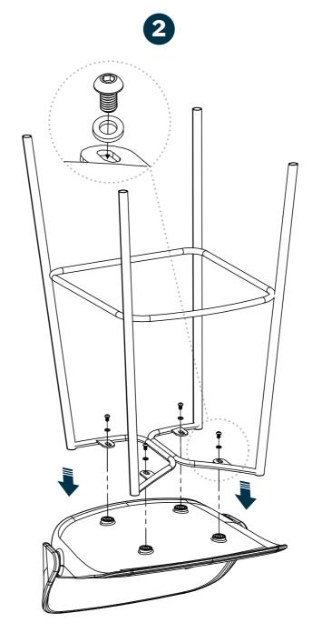
Use the hex key provided to securely tighten 4 screws and washers onto chair body.
