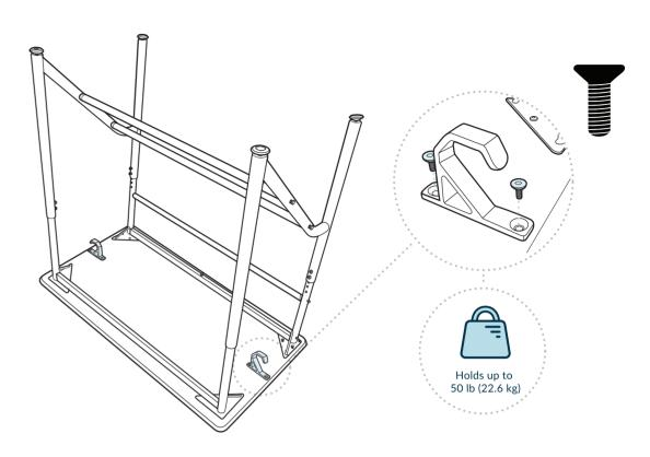
To install the bag hooks, line them up over the holes on each side of the desk between the legs and securely bolt them into place with the bolts pictured.
