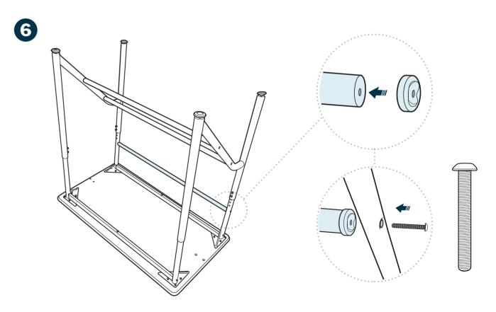
Add the smaller metal caps to the thinner crossbar and align with the holes towards the back of the desk. Attach the pictured bolts without fully tightening.
