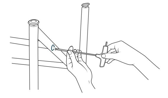
Go over each bolt connection and fully tighten using the Allen key to secure.
