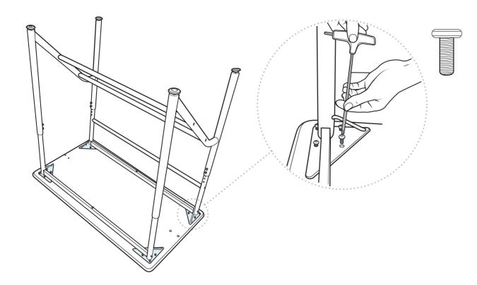
Now that the footrests and crossbar have been connected to the legs, you can fully tighten bolts into their brackets, using the Allen key to secure each bolt.
