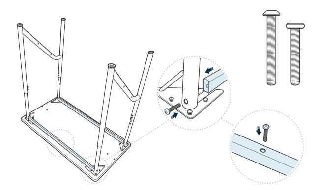
Place the long rectangular support bars in the bracket cutout. Attach the larger pictured bolts. Add the smaller pictured bolt into the middle of the support bar and fasten into the desk.
