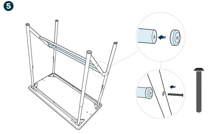
To install the 2 footrest bars, add the larger metal caps to each end of the bars, then line up with the leg holes. Attach the pictured bolts without fully tightening.
