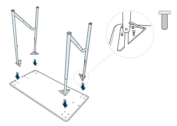
The desk leg brackets are marked with numbers 1 – 4. With the desk face side down, line up each leg with the corresponding number markers on the desktop corners. Attach the pictured bolts into the brackets without fully tightening.
