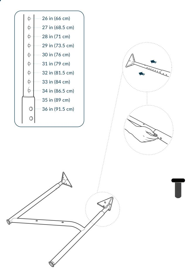
Pulling the tube through the metal leg, decide the height of the legs by aligning the holes and placing 2 of the pictured bolts into the holes without fully tightening. The legs can be adjusted to any height between 26" and 36" in 1" increments.
