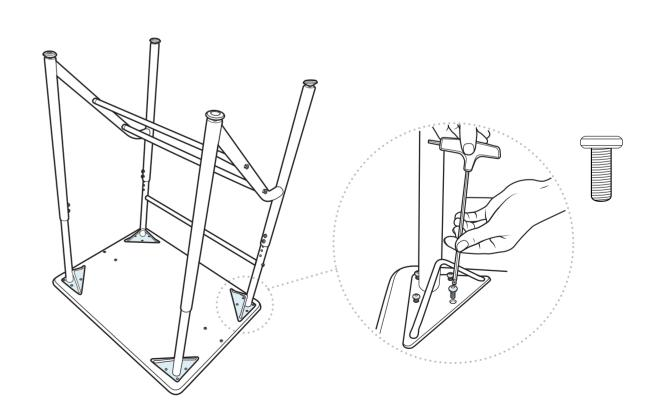
Now that the footrests and crossbar have been connected to the legs, fasten the 4 pictured bolts into the brackets.
