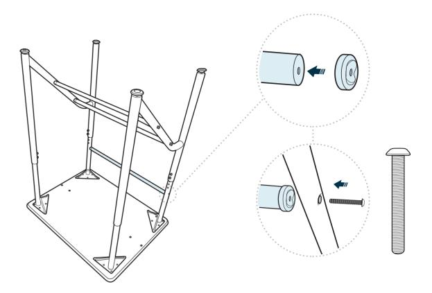
Add metal caps to the third, slightly longer bar and align with the holes towards the back of the desk. Attach the pictured bolts without fully tightening.
