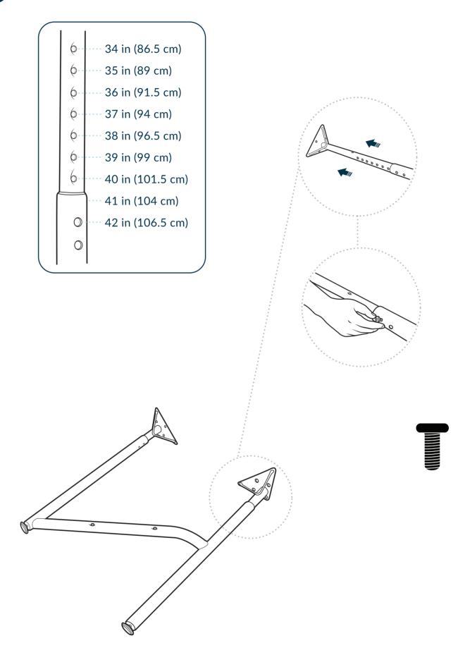
Pulling the tube through the metal leg, decide the height of the legs by aligning the holes and placing 2 of the pictured bolts into the holes without fully tightening. The legs can be adjusted to any height between 34" and 42" in 1" increments.
