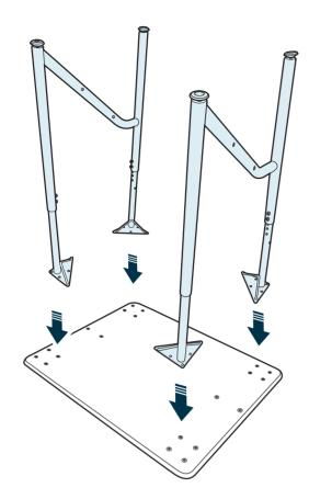
The desk leg brackets are marked with numbers 1 – 4. With the desk face side down, line up each leg with the corresponding number markers on the desktop corners.
