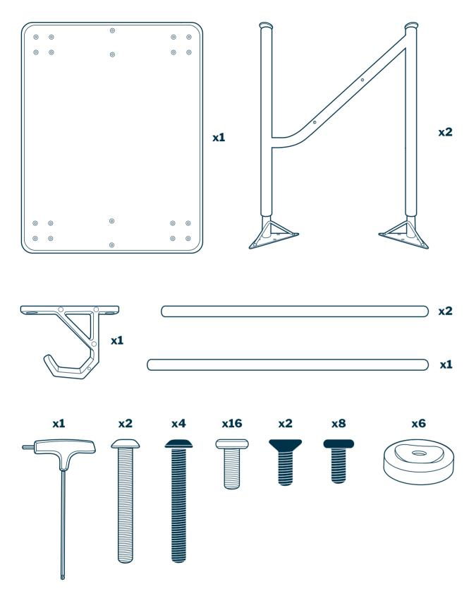
Remove everything from the box except for the desktop, placing the hardware bag of tools and bolts in an accessible area. Remove the legs from their plastic wrap.
