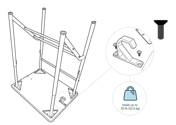
Install the bag hook to either side of the desk by lining it up over the holes on one side of the desk between the legs and securely attach with the 2 bolts pictured.
