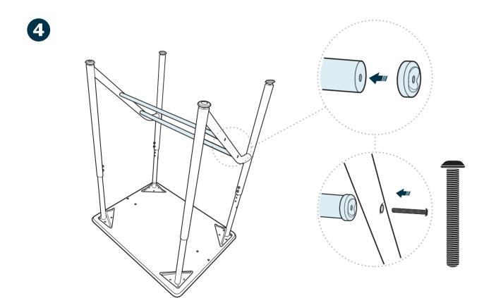
Take the 2 bars that are approx. 4 mm shorter, add the pictured metal caps to each end of the bars, then line up with leg holes. Attach the pictured bolts without fully tightening.
