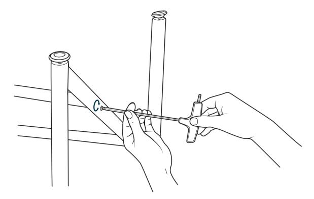
Using the Allen key, tighten each bolt connection until all are securely fastened.
