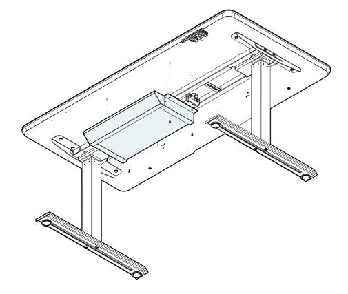
Hold the Desk Drawer in place while using 4 screws and the #2 Philips screwdriver (not included) to secure the Desk Drawer in the pilot holes.
