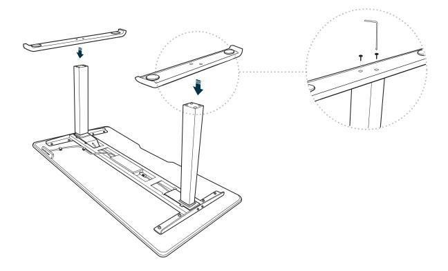
Once the control box is secure and while the desk is still face down, place one foot on top of one leg aligning the screw holes. Use the larger hex key (M10) provided to securely tighten screws (M10 - 40mm) into the feet. Repeat this step to attach the other foot.
