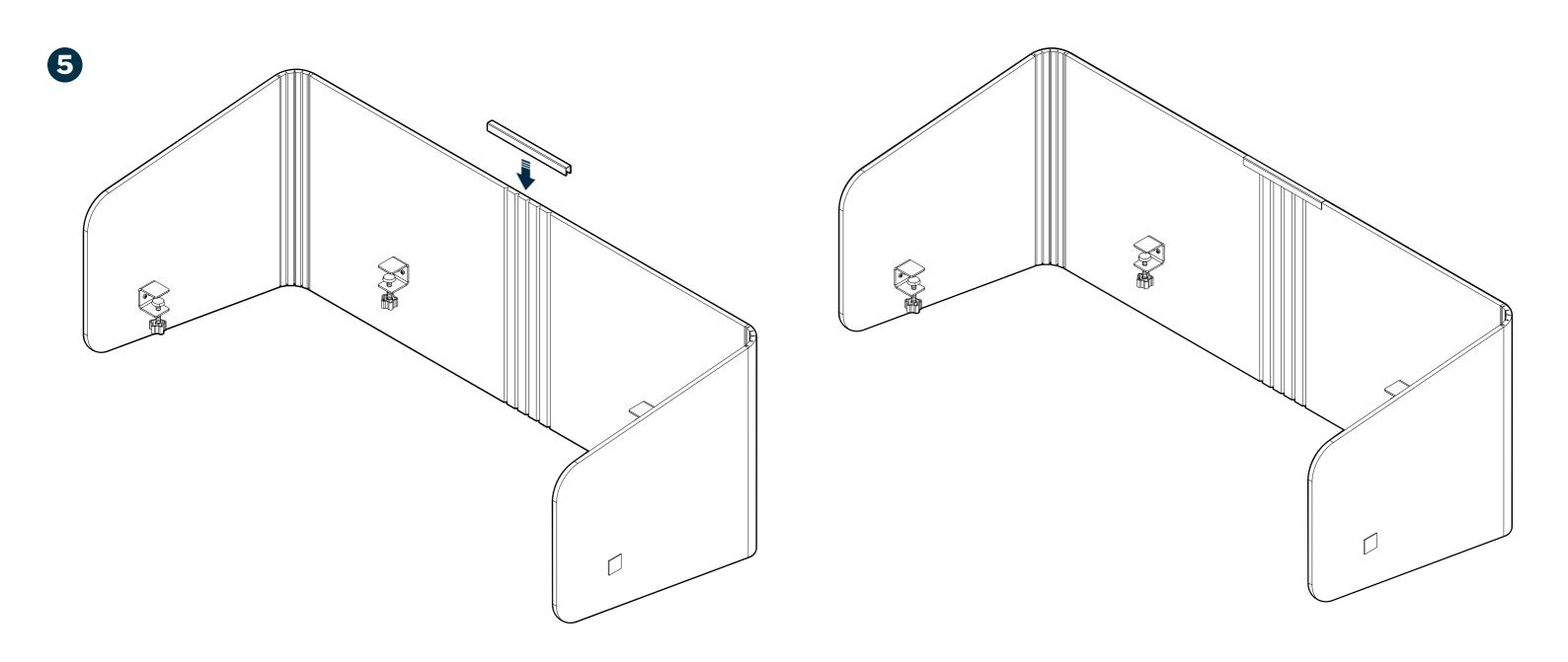
Slide the **CHANNEL COVER** onto the center of the **DESK SURROUND** to ensure it remains straight.
