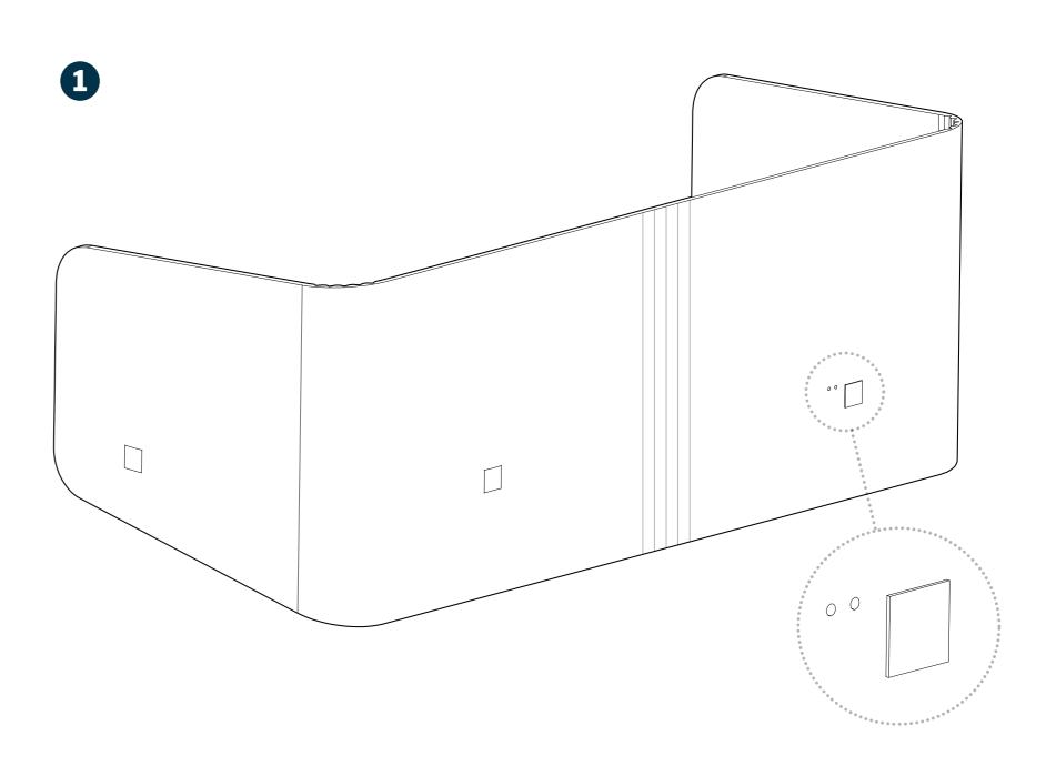
Remove the surround from the box and unfold it. Push the protruding edges of the **CLAMP PLATE** into the holes in the desk surround. Use two **CLAMP PLATES** on the back and one on each side.
