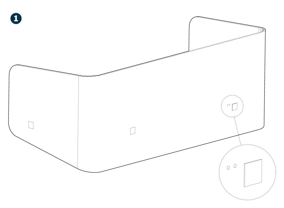
Push the protruding edges of the Clamp Plate into the holes in the desk surround. Use two Clamp Plates on the back and one on each side. Note: The Privacy Desk Surround is only compatible with Vari Electric Standing Desks 60" x 30" and 60" x 24".
