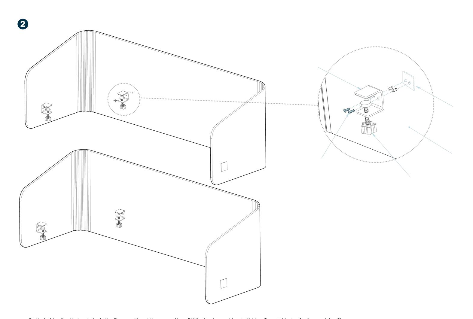
On the inside, align the two holes in the Clamp and insert the screws. Use a Phillips head screwdriver to tighten. Repeat this step for the remaining Clamps
