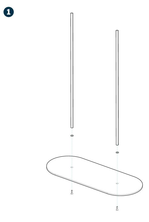
Insert the screws through the base plate, thread the washer on and screw into the metal rods. You can use a 5 mm Allen key to tighten the screw.
