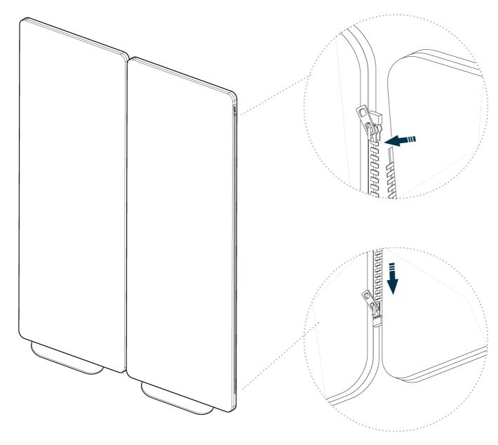
The Privacy Screen Panels can be used as freestanding panels or combined to create a panel system. If you are assembling it as a panel system, align the zipper ends and zip down to connect panels.
