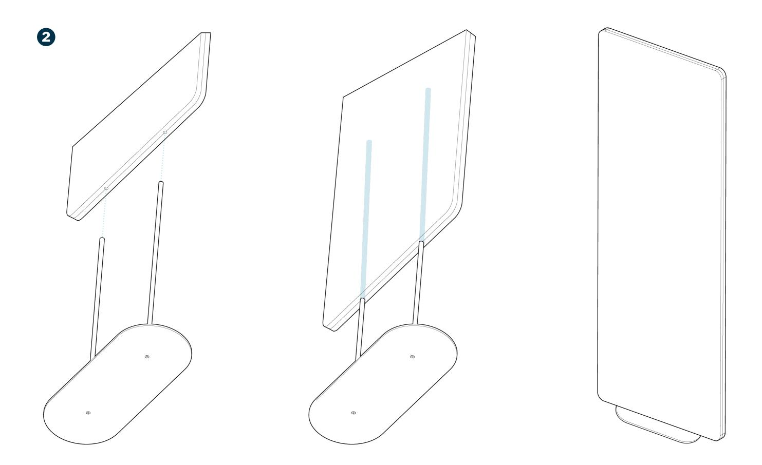
Align the holes in the bottom of the screen and slide the rods in until the panel touches the base plate.
