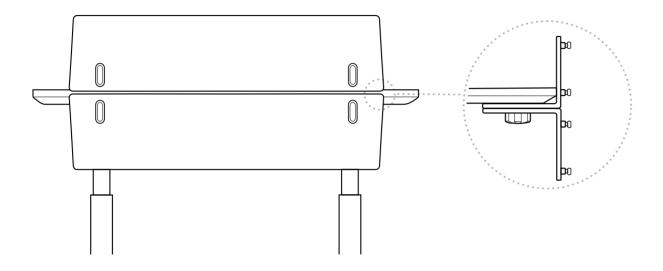
To use both panels and create a privacy and modesty panel setup, put one upward facing bracket on top of a downward facing bracket.
