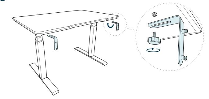
To attach the brackets, put the bolt through the bracket cutout. Find the pre-drilled holes located underneath the desk near the cable tray. Attach the bracket to the desk using the included hand bolt. Do not fully tighten.
