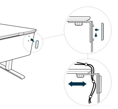
Press the bracket covers onto the front and pull down. Adjust the panel as needed to accommodate cords or desk items. Fully tighten the bolts once the panel is in
