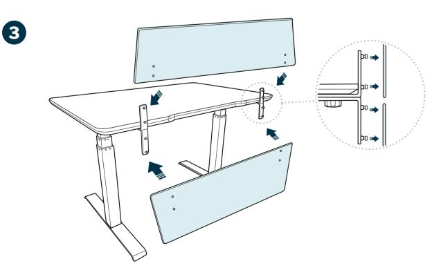
One at a time, align the holes of each panel with the front of each set of brackets. Push each panel onto the brackets on each side.
