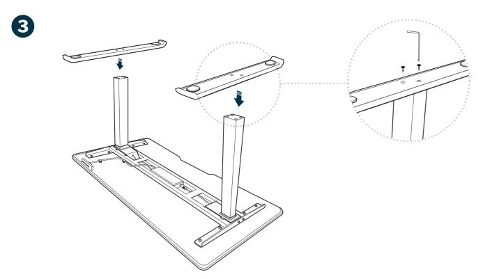
Once the control box is secure and while the desk is still face down, place one foot on top of one leg aligning the screw holes. Use the larger hex key (M10) provided to securely tighten screws (M10 - 40mm) into the feet. Repeat this step to attach the other foot.
