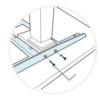
Use the smaller hex key (M6) provided to securely tighten the screws and washers (M6 - 14mm) onto each leg.
