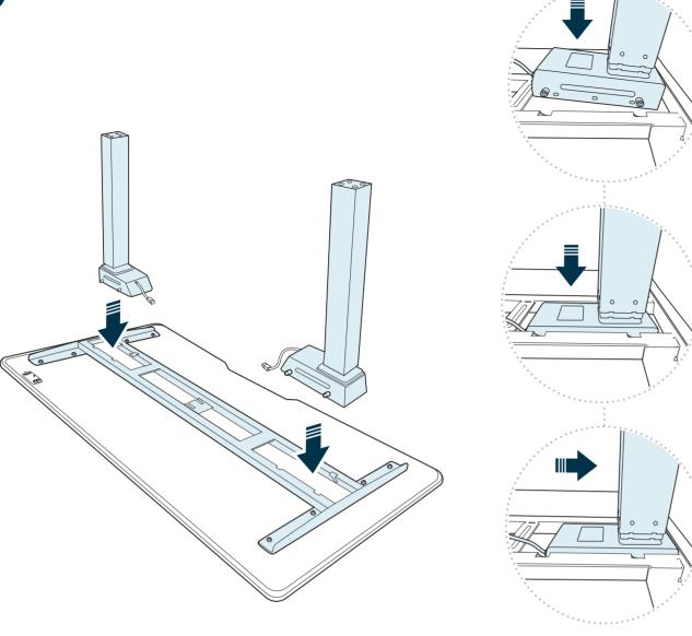
Desktop and desk legs will arrive in separate boxes. We recommend assembling the desk with the desktop face down in the box to prevent any surface scratching. Open the desktop box. Remove the desk legs from their box.
