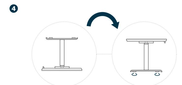
Once legs and feet are secure, two people should carefully flip the assembled desk (along the back edge to avoid damaging the control panel) to an upright position. Adjust the footpads to level the desk as needed.
