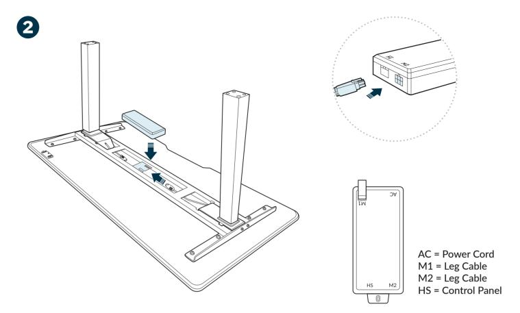
Once the legs are secured with screws and while the desk is still face down, lower the control box into the middle cavity of the metal frame. Then, slide the control box to engage the bracket that holds the control box in place. When the control box is secured, connect the leg cables to the corresponding control box inputs, M1 and M2.
