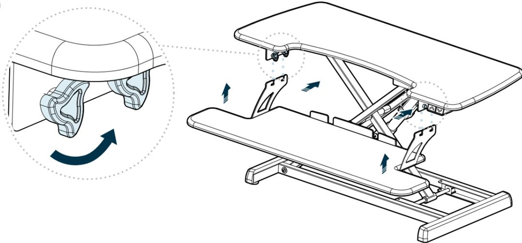
Locate the 4 pre-installed handscrews below the top tier. Loosen each of the handscrews, using one hand to hold one end still while turning the other end, until the post in between ends is accessible. Align the notches on the keyboard tray brackets with the handscrew posts, then slide the keyboard tray into place in an up-and-back motion. Tighten each of the handscrews to secure the tray in place.
