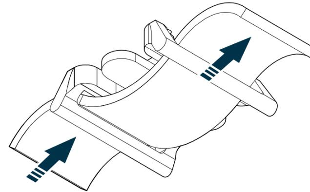
Push the velcro strap into the slots of the bracket.
