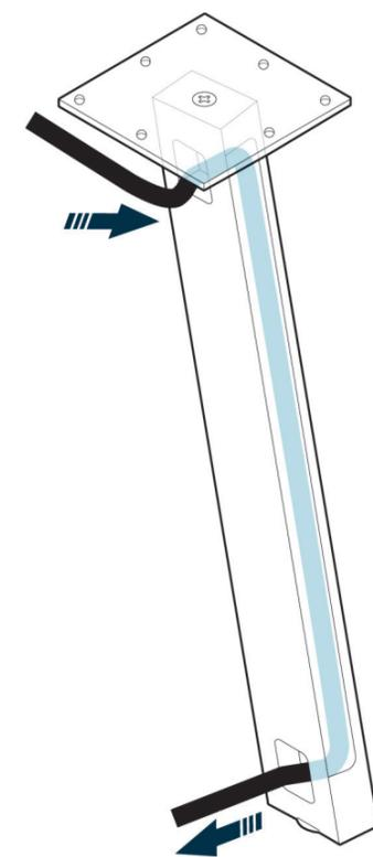
Unroll and relax the kinks in the power cord. Then, run it down the cable management slot provided in the proper alternate leg.
