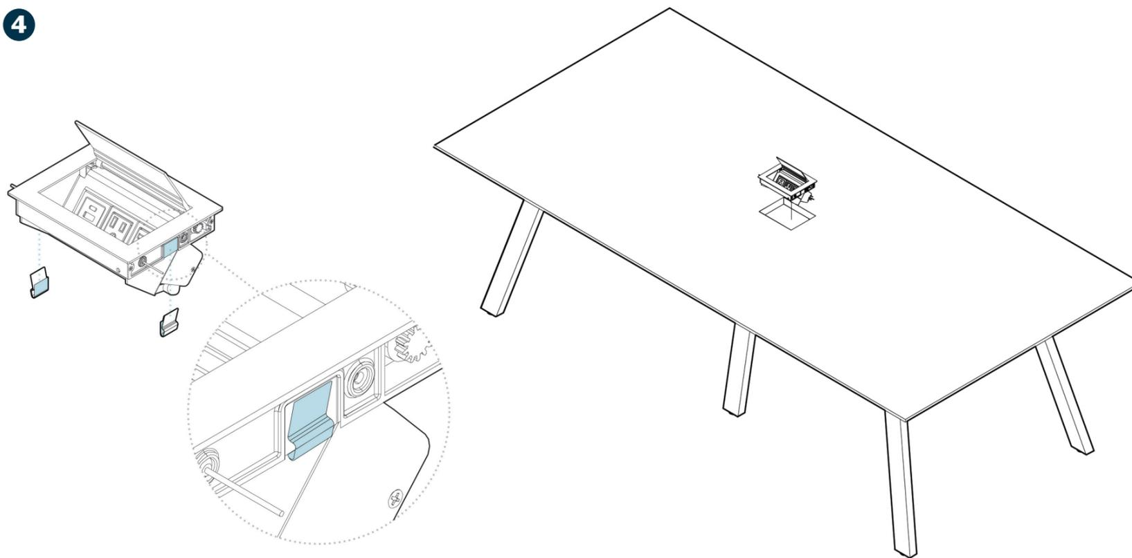
Slide the clips onto the right and left side of the power box, place it into the center of the tabletop, and press down to firmly secure them. The power unit is installed properly when it is flush with the tabletop surface.
