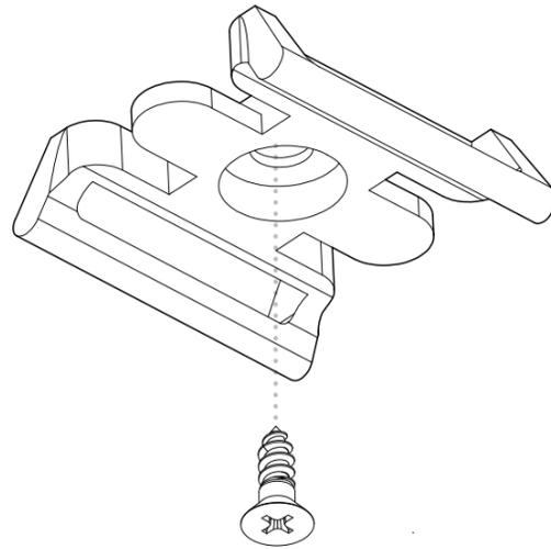
Screw the bracket into the underside of the table, in the path of the cable.
