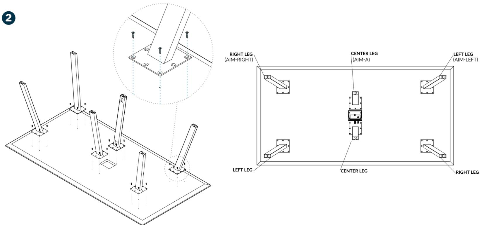
The left, right, and alternate legs are labeled on the plate of each leg. (Center legs are labeled "AIM-A" and one should have a cutout for cable management). Align the square plate at the top of each leg with the corresponding pre-drilled holes on the underside of the tabletop. Use the provided screws and your Phillips Head screwdriver to secure them to the table, one by one.
