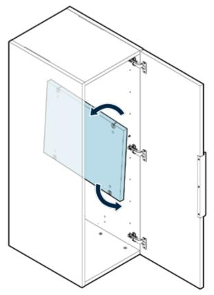
Separate the shelf from the mini fix cams (either by lifting the shelf if the mini fix cams were on the bottom, or by gently lowering it if they were on top), then rotate the shelf onto its side.
