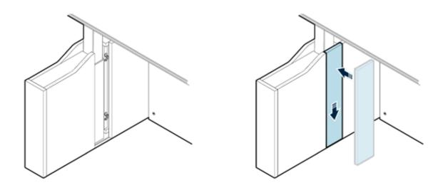
Reinstall the panel on the inside of the left base by aligning it with the base opening and lowering it into place until the pegs catch on the latches.
