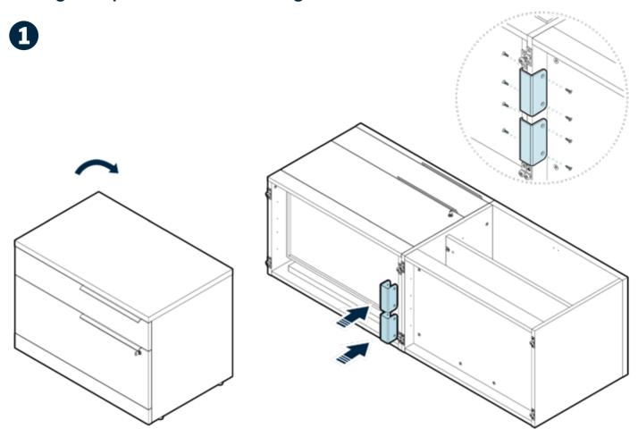
With assistance, tilt the empty lateral file cabinet onto its back, and position it side-by-side with the other piece(s) of furniture. Slide two joining brackets over the adjacent side panel bases, aligning the holes in the brackets with the holes in the panels. Using a Phillips head screwdriver, secure each bracket with four wood screws.
