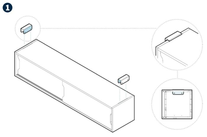
Overhead cabinets can be installed between two wardrobe cabinets to sit on top of a 96" lower credenza. Lower one side of a joining bracket into a slot on top of the overhead cabinet. Using a Phillips head screwdriver and two of the provided wood screws, attach the bracket to the inside of the overhead cabinet. Repeat for the second end.
