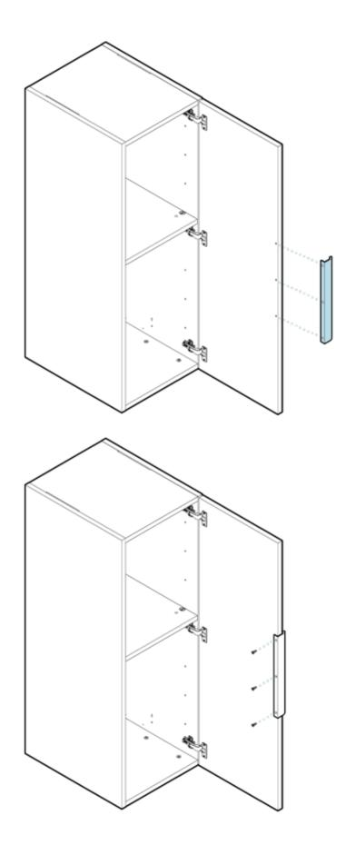
After the door orientation has been determined, the door pull can be attached. Align the door pull to the predrilled holes on the cabinet door, and secure the pull with the 3 #8 x %" Phillips head screws and a Phillips head screwdriver.
