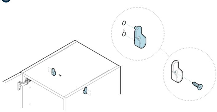
Open the wardrobe cabinet. Align a rail support with the predrilled holes near the top of the cabinet, then push the pegs on the back of the support into the holes. Using a Phillips head screwdriver and 1 of the provided  $\#8 \times \%$ " Phillips head screws, secure the rail support in place. Repeat for the opposite side of the cabinet.
