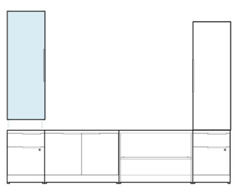
With assistace, tilt the cabinet onto its back edge, then lift it up. Carefully hover the cabinet over the lower cabinets. (NOTE: If installing on a credenza of joined cabinets, the credenza should be 96" wide and already in its final arrangement.) After ensuring all back and side panels are flush with each other, lower the cabinet into place.
