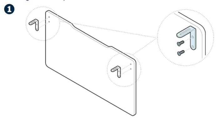
Attach the brackets to the modesty panel using the four provided M5 flathead screws and a Phillips head screwdriver.
