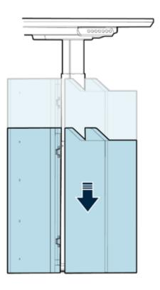
Slide the open right base around the right leg, then lower it into place over the right foot.
