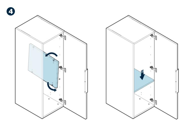
Rotate the shelf until it is horizontal with the mini fix cams facing down, then lower it onto the pegs. Use a Phillips head screwdriver to turn each mini fix cam clockwise, locking the shelf in place.
