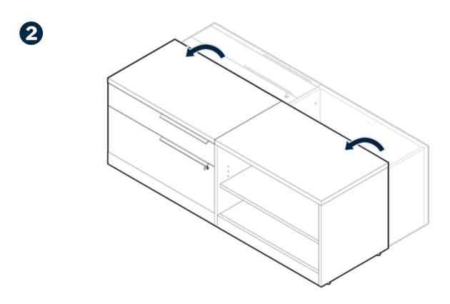
With assistance, tilt the joined pieces onto their feet. Use a ½" wrench to level as needed.
