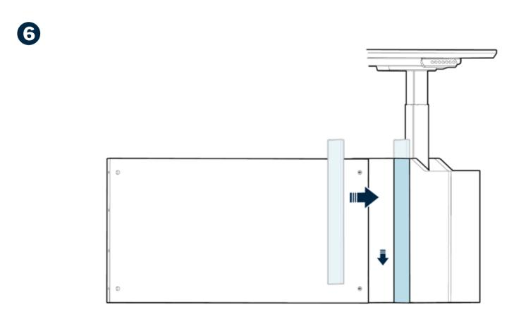
Reinstall the panel on the inside of the right base by aligning it with the base opening and lowering it into place until the pegs catch on the latches.
