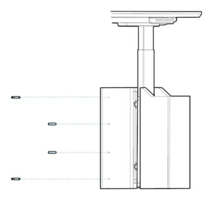
Insert two of the dowels into the middle two holes on the right base. Then, using a Phillips head screwdriver, screw in two of the mini fix studs into the top and bottom holes.
