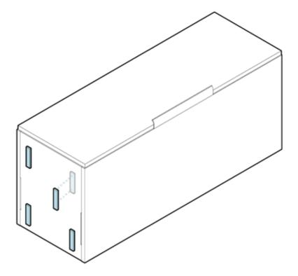
With assistance, tilt the wardrobe cabinet onto its back. Remove the backing from one side of the provided 4" pieces of VHB tape, and apply it to one of the 4 corners of the bottom panel. Repeat with the remaining 3 pieces. With all 4 pieces applied to the wardrobe cabinet, remove the backing from the exposed side.
