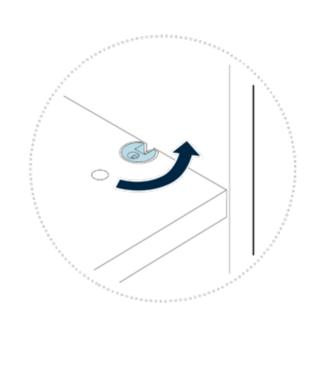
NOTE: The shelf should only be used with the mini fix cams face-down. If the cabinet was rotated to switch the door's orientation, the shelf will need to be removed and flipped.
