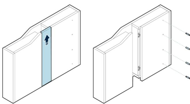
Remove the panel on the inside of the left base, sliding it up to release it from the latches. Insert two of the dowels into the middle two holes on the left base. Then, using a Phillips head screwdriver, screw in two of the mini fix studs into the top and bottom holes.
