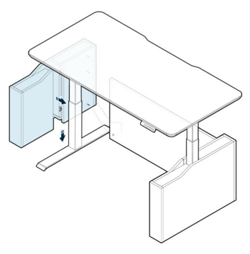
Slide the left base around the left leg of the desk, then lower it into place over the left foot of the desk. Make sure to line up the dowels and mini fix studs with the holes on the lower panel.
