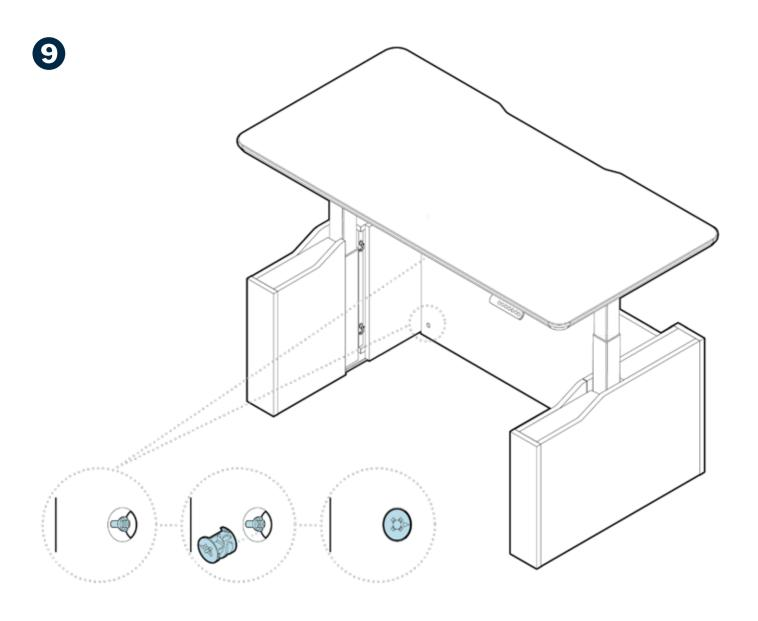
The mini fix studs should be visible in the holes. Insert the mini fix cams into the holes, with the arrows facing the left base. Once the mini fix cams are flush with the panel, use a Phillips head screwdriver to turn them until the arrows face away from the left base.
