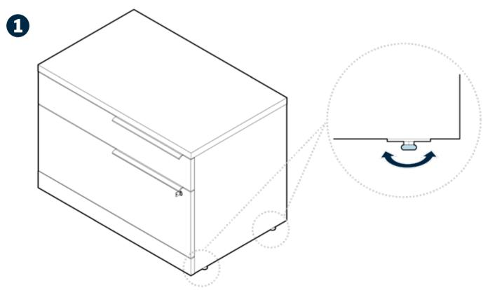
To adjust the leveling foot under each corner of the lateral file cabinet, use a ½" wrench to twist each foot as needed. Turning the wrench clockwise lowers the foot, while turning the wrench counter-clockwise raises it.
