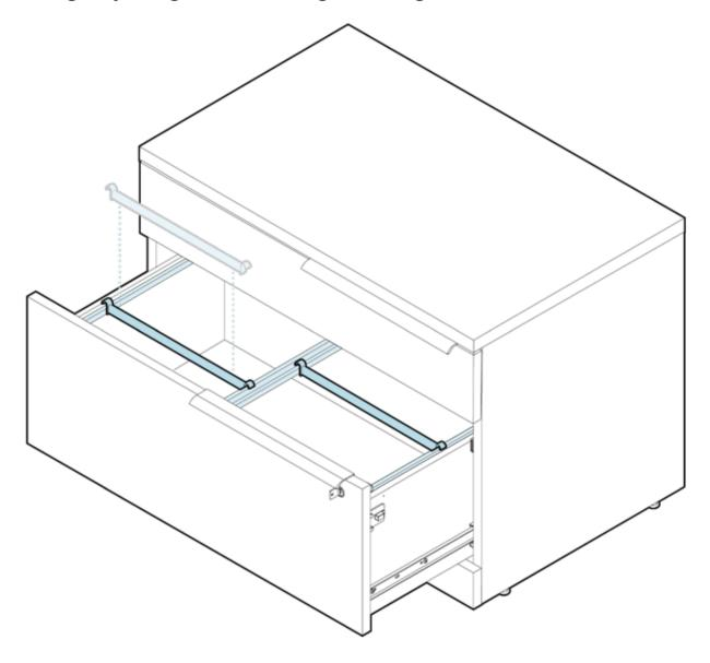
The lateral file cabinet will come with 5 file rails—4 long and 1 short. These can be lowered into place, resting front-to-back or side-to-side on other supporting track. To reposition or remove the file rails, press along the bottom of the supporting track near the file rail to release the locking tooth, then slide the rail into the desired position or lift the rail off the tracks to remove.
