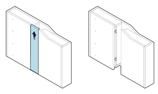
To remove the panel on the inside of the right base, slide it up to release it from the latches.
