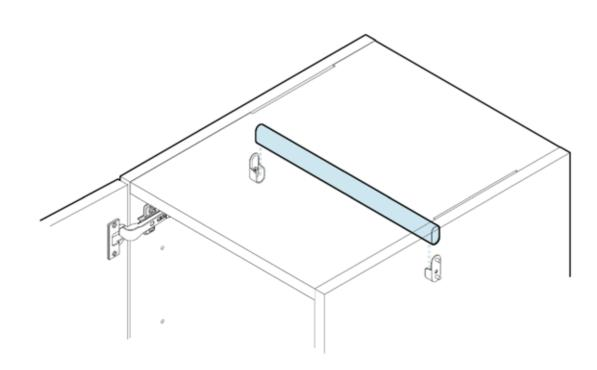
Align the clothing rail with the rail supports and lower into place. Tug firmly on the rail to ensure it is securely installed.
