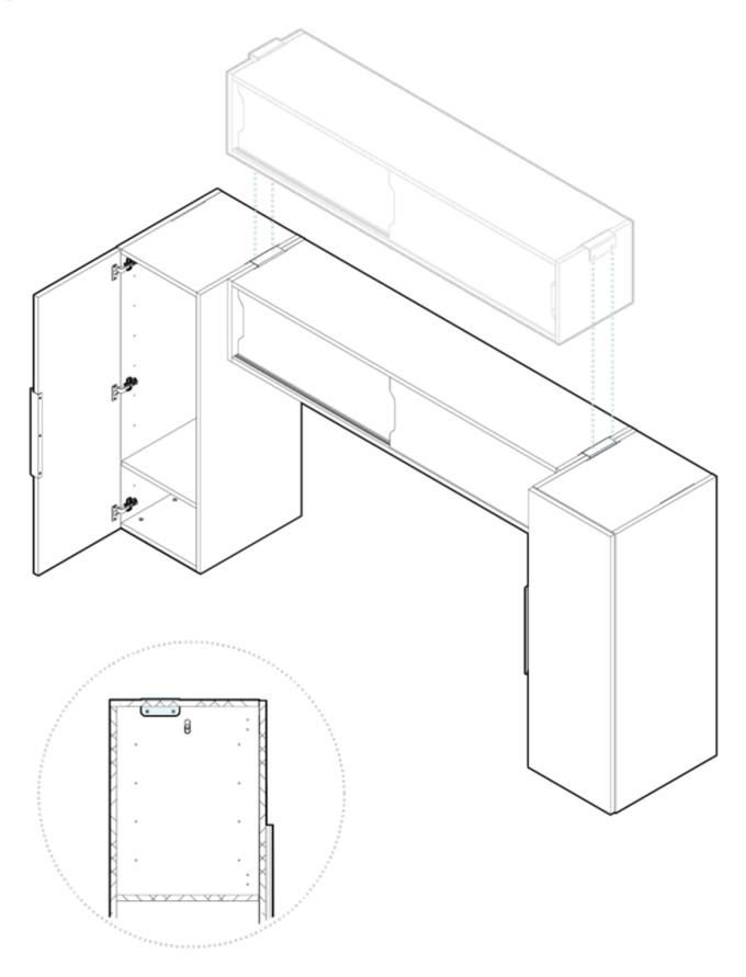
With assistance, carefully lower the overhead cabinet onto two wardrobe cabinets, with the joining brackets sliding into the slots on top of the wardrobe cabinets.
