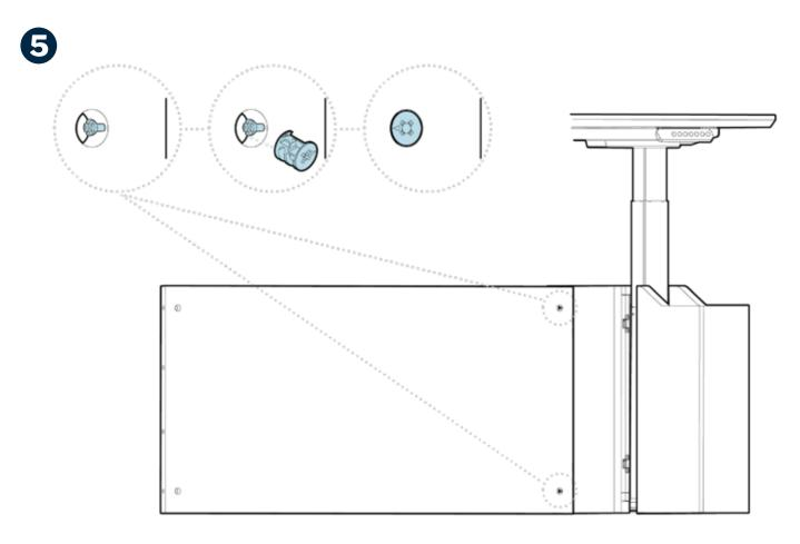
The mini fix studs should be visible in the holes. Insert the mini fix cams into the holes, with the arrows facing the right base. Once the mini fix cams are flush with the panel, use a Phillips head screwdriver to turn them until the arrows face away from the right base.
