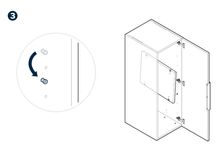
Move each peg to the desired position, confirming that all four pegs are on the same level.
