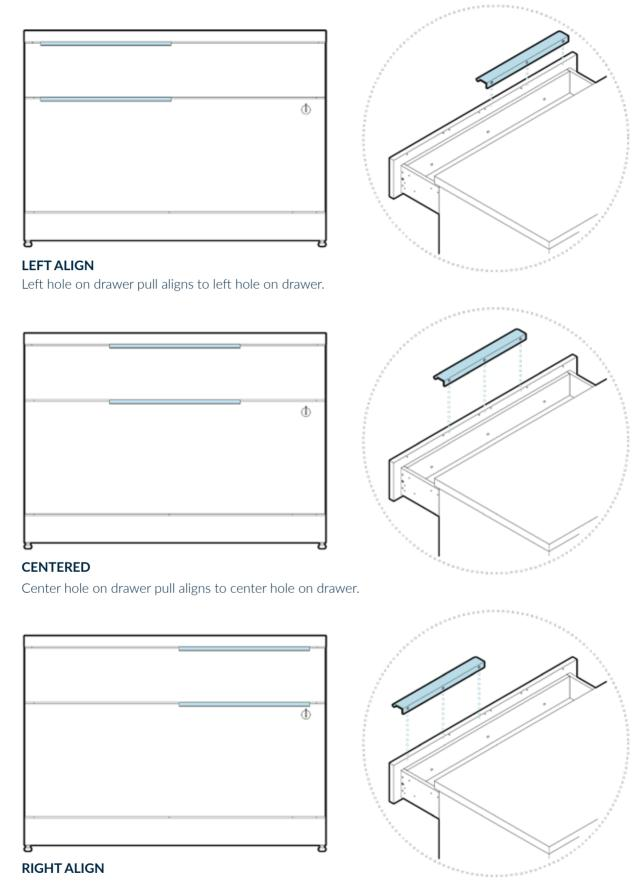
Right hole on drawer pull aligns to right hole on drawer.
