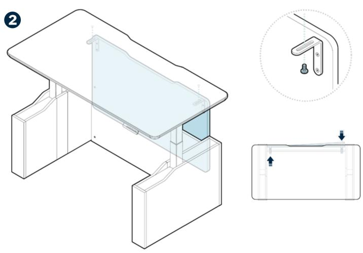
With assistance, lift the panel to the bottom side of the desk, aligning the panel's brackets with the insert nuts on the bottom of the desk. Thread the M8 pan head screws through the bracket openings, and secure them to the desk using a Phillips head screwdriver. Be sure the panel is straight and not hitting the lower panel; if adjustments are needed, loosen the screws, slide the bracket into the desired position, and retighten. Confirm the panel is secure before use.
