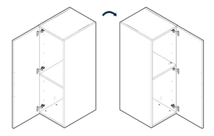
Before installing the cabinet, determine the direction you want the door to open. Then, if needed, rotate the cabinet so that the door opens in the desired direction.
