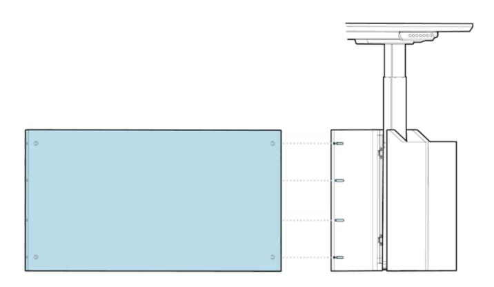
Slide the right end of the lower modesty panel onto the dowels and mini fix studs.
