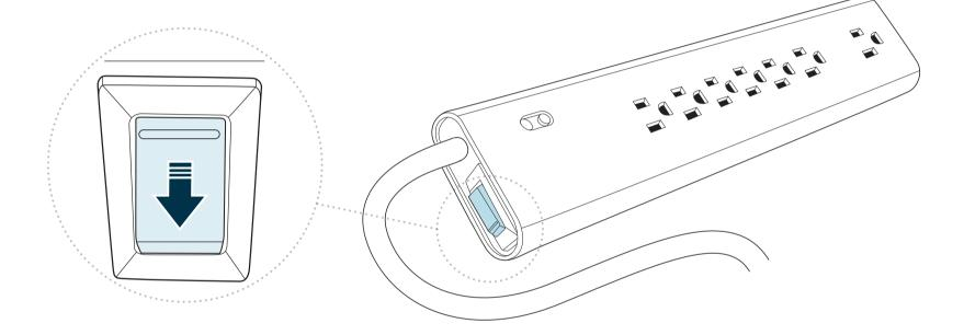
Plug directly into a grounded outlet - do not plug into a power strip. Press switch towards "reset" on side of strip to turn on. Green and red lights will be lit when the power strip is on, indicating that it's protected and grounded.
