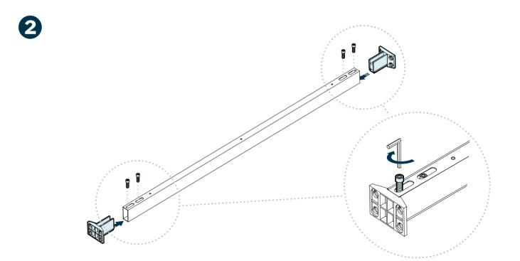
Secure the connecting brackets to the support bar using four (4) M8-20 Screws and the M4 Allen key. If assembled correctly, the surface of the bar should be flush with the surface of the bracket, not offset.
