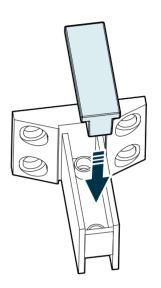
Assemble the connecting bracket by placing the bracket cover over the insert nuts as shown above (note the orientation of the connecting bracket). Repeat the step for the second bracket.
