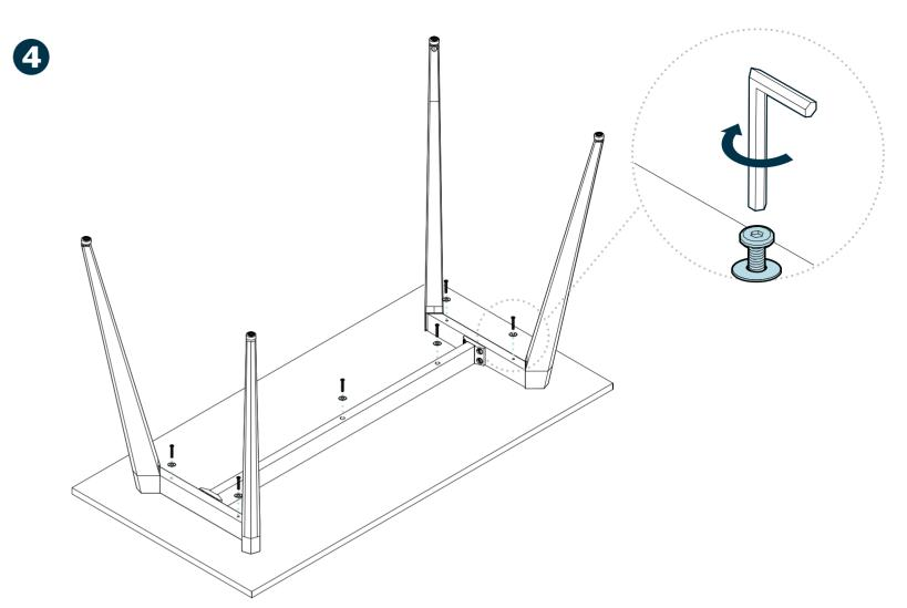
Next, attach the assembled legs and support beam to the desk top using seven (7) of the M6-65 screws, seven (7) of the M6 washers, and the M6 Allen key.
