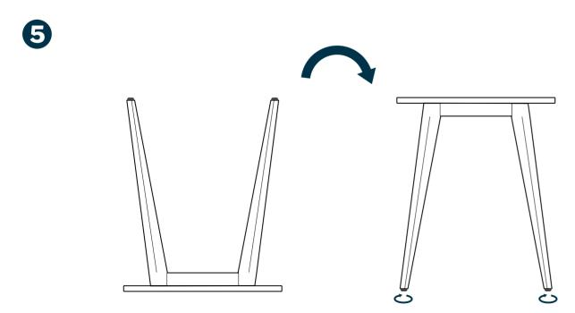
Using two people, lift and turn the desk over, and set it down gently on its feet. Adjust the footpads to level the desk as needed. Your desk is now completely assembled and ready to use.
