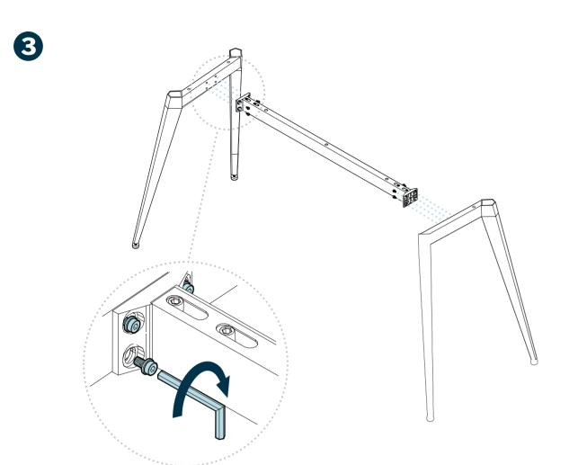
Using two people, attach the support beam assembly to the legs using eight (8) M6-16 screws and the included M5 Allen key as shown above; the side of the beam with more holes should be positioned to face the bottom of the desk top. **Do not tighten completely.**
