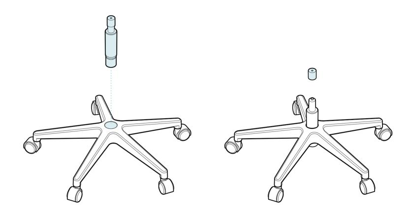
Place the piston into the center of the base with the smaller end pointed up. Remove the piston cap cover.
