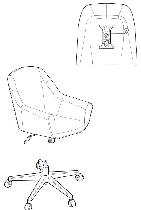
With assistance, take the chair seat and place the highlighted section of the mechanism onto the highlighted section of the piston.
