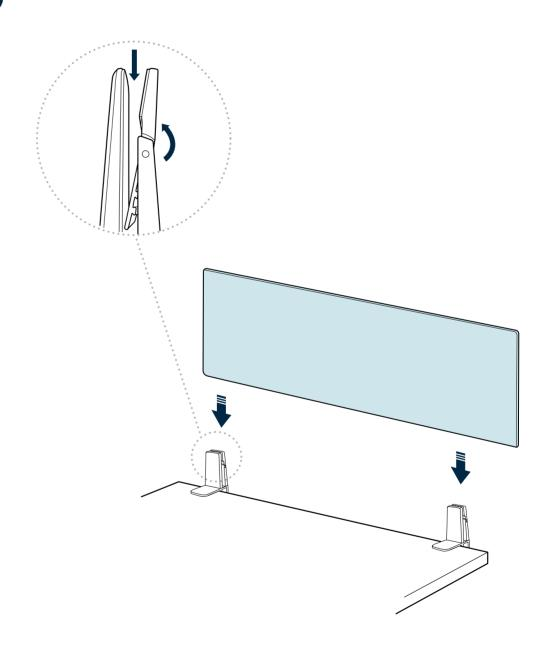
Carefully slide the acrylic panel all the way down into the brackets.
