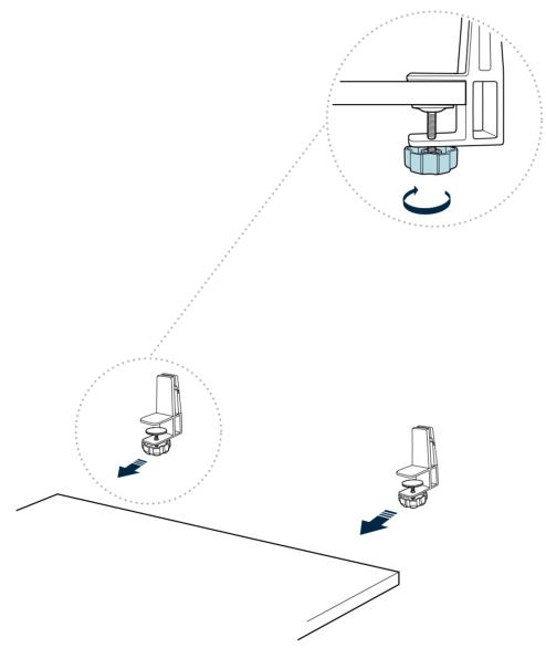
Turn the hand bolts counterclockwise to open the clamp. Position each clamp at about the same distance in from the front and back of the desk (or table), then slide the clamps onto the end of the desk. Turn the hand bolts clockwise to tighten them.
