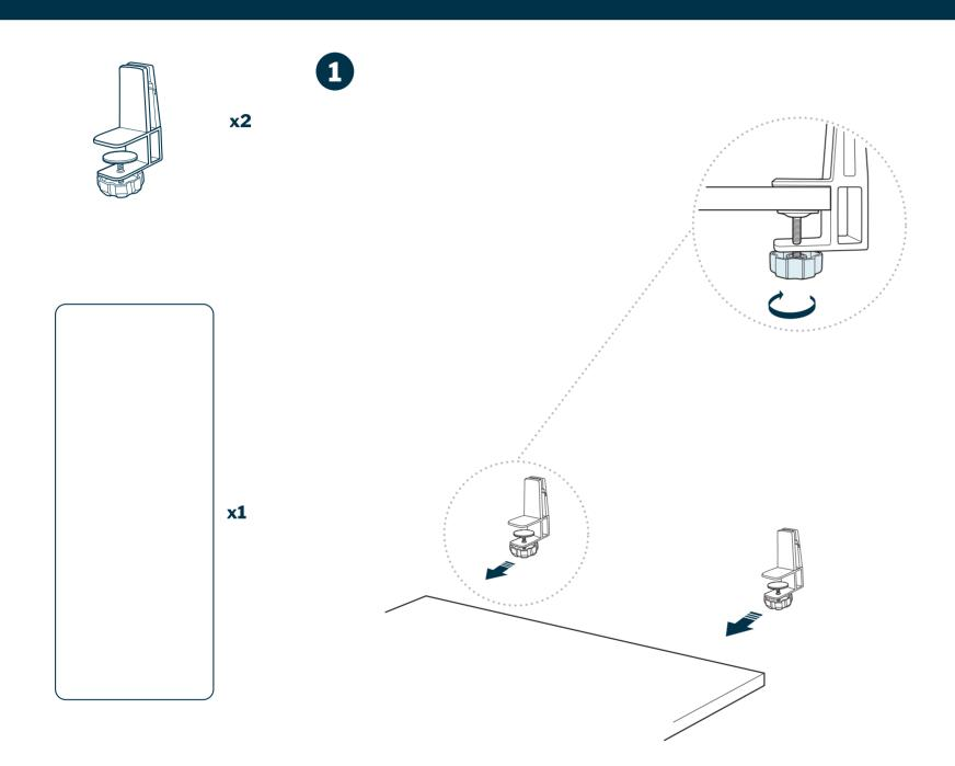
Position each clamp at about the same distance on the side of the desk. Slide the clamps onto the edge of the desk and tighten them using the hand bolts.
