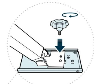
Once you've selected your preferred height setting, use the hand bolts to secure and tighten the legs into place. Remove the cardboard guides.
