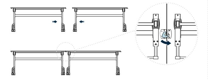
To link multiple tables together, line them up side-by-side facing the same direction. Once in place, rotate the latch hook on the underside of one table through the latch on the underside of the second table.
