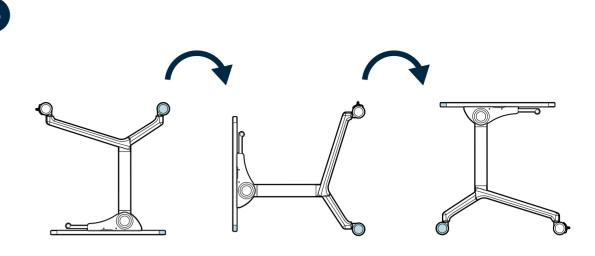
To insert the casters, first line up the casters that have a lock (a) with the longest feet closest to the locking mechanism and press down until the caster is flat against the foot. Then, line up the casters that do not have a lock (b) with the shortest feet and again press down until the caster is flat against the foot.
