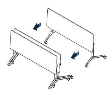
When the Flip Top Training Table is in the upright position, multiple tables can be nested together for storage. Position the tables to face the same direction, align each end, and push them together, carefully guiding the legs of the back table between the legs of the front table.
