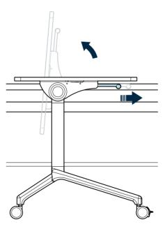
With two hands, pull and hold the locking mechanism out toward the table edge, then tilt the table top into the upright position. Once it is in place, release the locking mechanism.
