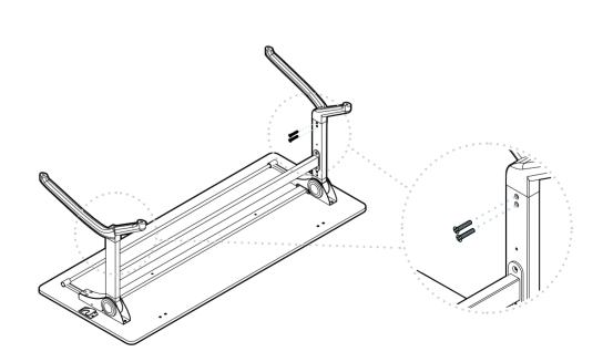
Following the "L" (left) and "R" (right) indicators on the feet and the interior side of the legs, insert the feet into the corresponding legs of the table. Using a Phillips screwdriver and the included screws, secure both feet in position. If you purchased a modesty panel, please refer to the separate instructions included with the modesty panel before moving on to the next step.
