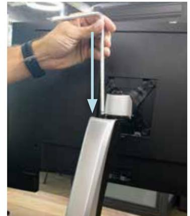
If your monitors are popping up too high, you want to loosen the tension by turning the wrench counter-clockwise toward the “-” symbol.
