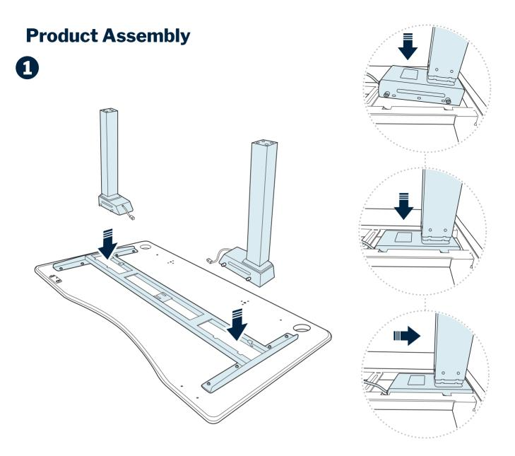
Desktop and desk legs will arrive in separate boxes. We recommend assembling the desk with the desktop face down in its box to prevent any surface scratching. Open both boxes; remove the desk legs and parts from their box.
