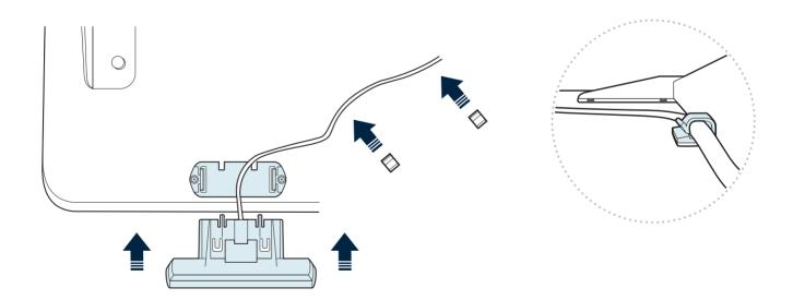
Locate the control panel and slide it into the bracket to attach. Once the panel is in place, connect its cable to the corresponding control box input, HS.
