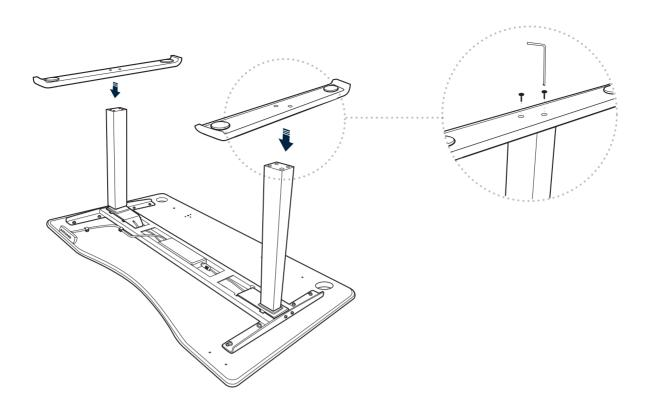
Once the control box is secure and while the desk is still face down, place one foot on top of one leg aligning the screw holes. Use the larger hex key (M10) provided to securely tighten screws (M10 - 40mm) into the feet. Repeat this step to attach the other foot.
