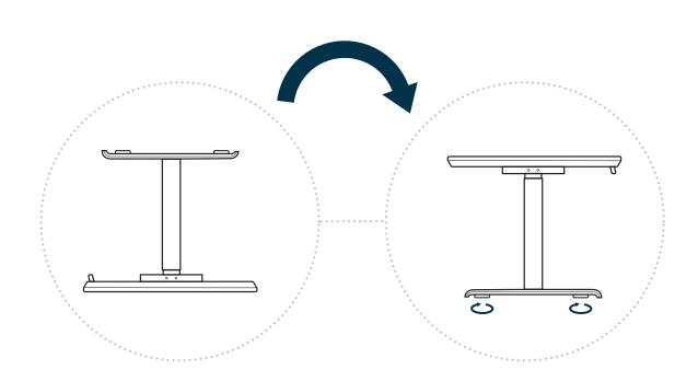
Once legs and feet are secure, two people should carefully flip the assembled desk (along the back edge to avoid damaging the control panel) to an upright position. Adjust the footpads to level the desk as needed.
