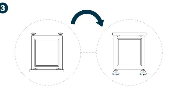
Two people should lift and flip the assembled table to an upright position. Adjust the footpads to level table as needed.
