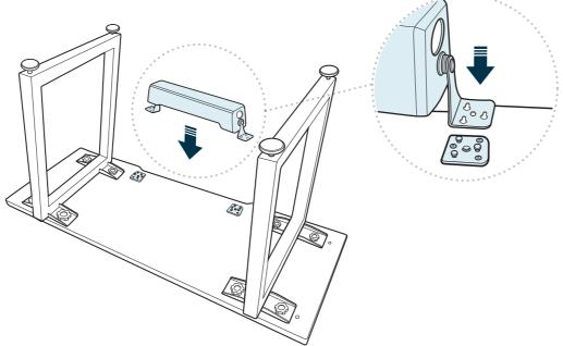
Slide the cable management tray into the notches at the edge of the table and push until it clicks, indicating it is locked into place.
