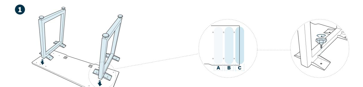
Table top and table legs will arrive in separate boxes. We recommend assembling the table face down in the box to prevent any surface scratching. Unbox the legs and line up legs with desired connection points.
