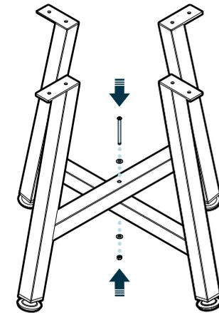
Place the spacer on top of the base leg crossbar, and make sure it drops into place. Then, place the top leg on the spacer, lining up the holes. Line up the bolt, washers, and nut in order to sandwich the legs and hold everything in place. Using the wrench to hold the nut still, turn the bolt with the Allen Key until tightly fastened.
