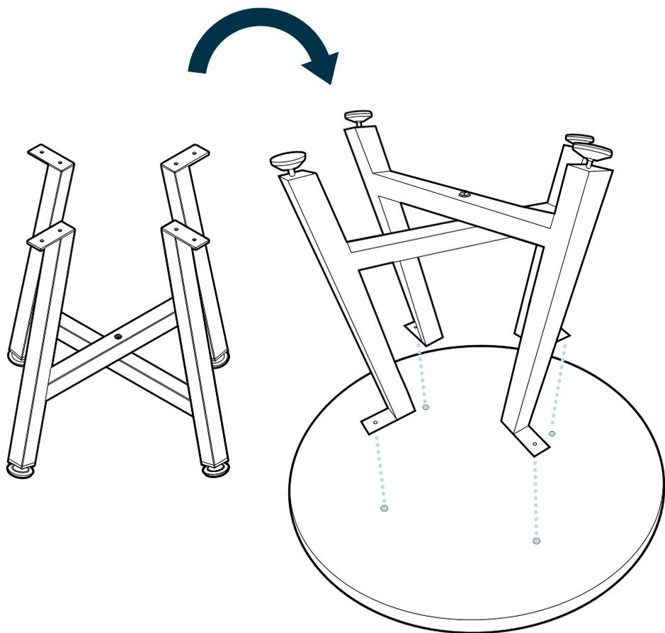
**NOTE: We recommend assembling the table face down in the box to prevent any surface scratching.**
