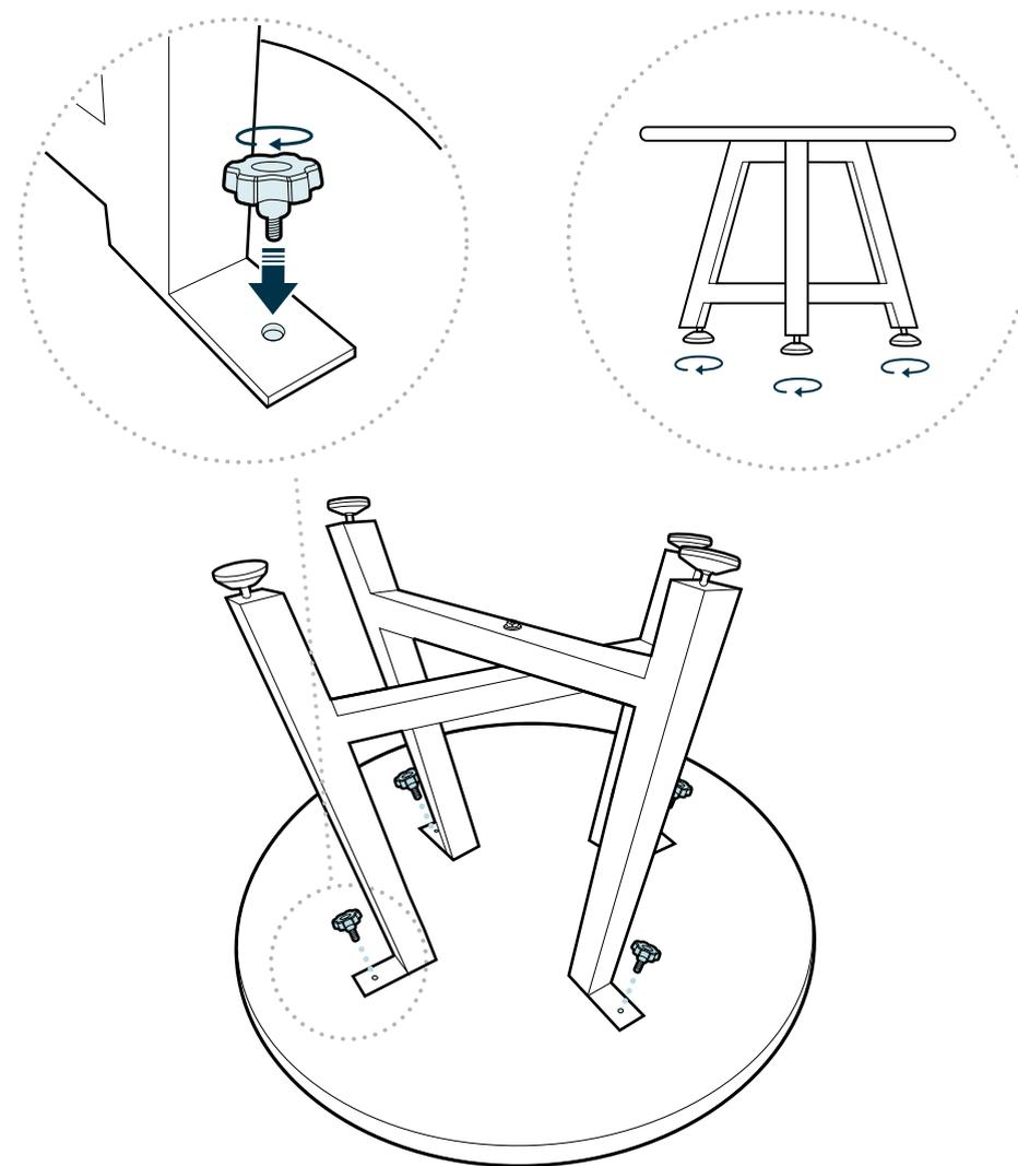
Use the hand bolts to fasten the legs to the table top, and tighten until firmly in place. With the assistance of another person, lift and flip the assembled table to an upright position.
