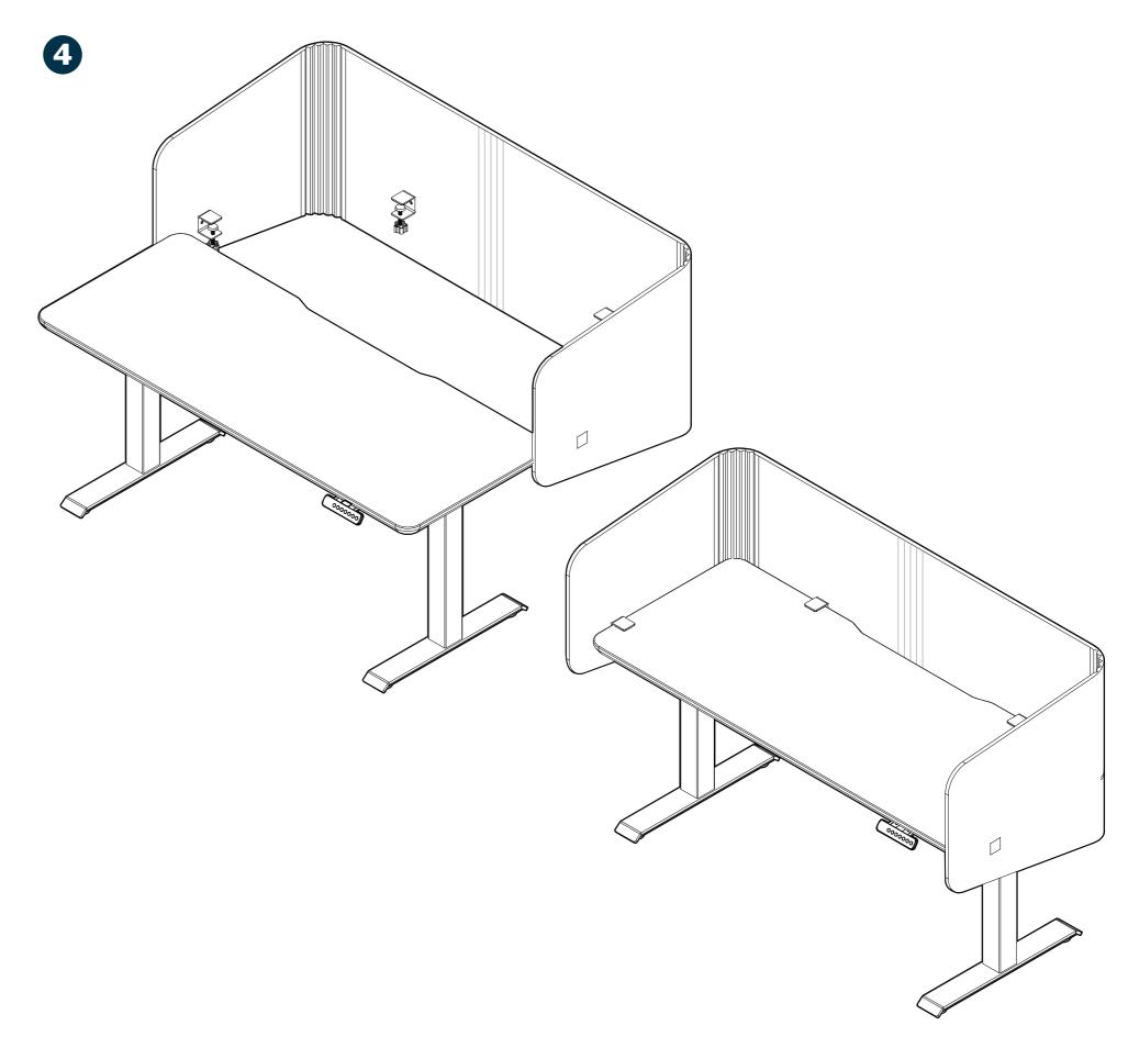
Slide the Clamps onto the edge of the worksurface and turn the knobs to secure the Desk Surround to the desk.
