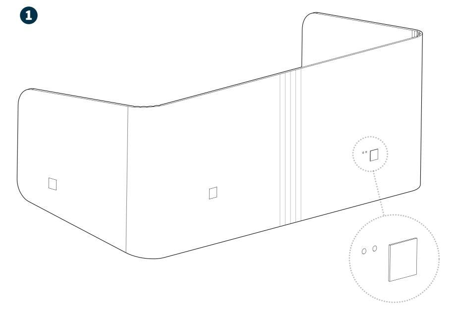
Remove the surround from the box and unfold it. Push the protruding edges of the Clamp Plate into the holes in the desk surround. Use two Clamp Plates on the back and one on each side. **Note: The Privacy Desk Surround** and **Tall Privacy Desk Surround** are only compatible with **Vari Electric Standing Desks 60"** x 30" and 60" x 24".
