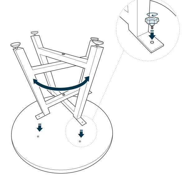
Table top and table legs will arrive in separate boxes. We recommend assembling the table face down in the box to prevent any surface scratching. Unbox the legs, pull apart to create an "X" with the frame, and line up with table top connection points. Use the hand bolts to fasten the legs to the table top and tighten until firmly in place.
