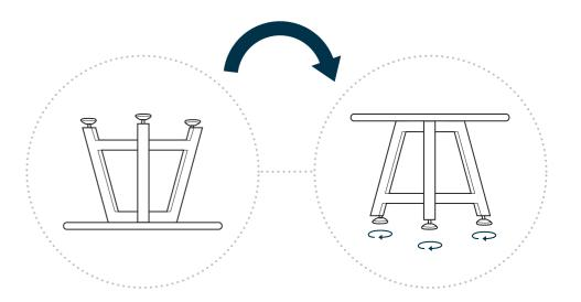
Two people should lift and flip the assembled table to an upright position. Adjust the footpads to level the table as needed.
