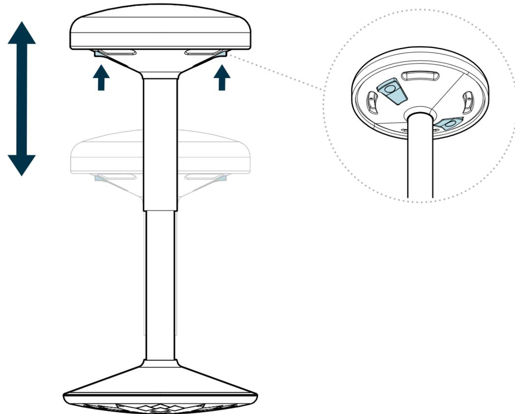
To raise or lower the seat, press and hold one or both buttons under the seat cushion, and release when the stool is at the desired height.
