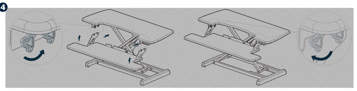
Locate the 4 pre-installed handscrews below the top tier. Loosen each of the handscrews, using one hand to hold one end still while turning the other end, until the post in between ends is accessible. Align the notches on the keyboard tray brackets with the handscrew posts, then slide the keyboard tray into place in an up-andback motion. Tighten each of the handscrews to secure the tray in place.
