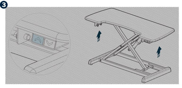
With the converter plugged in, press the up arrow button until the converter is raised to its highest position, providing room to attach the keyboard tray.
