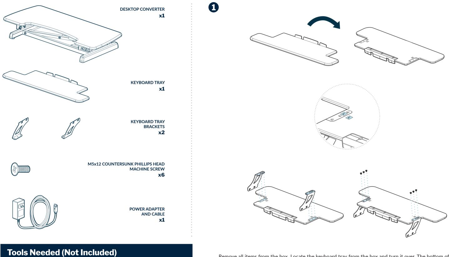
Remove all items from the box. Locate the keyboard tray from the box and turn it over. The bottom of the tray and the keyboard tray brackets will be marked with L and R stickers. Align each bracket with its corresponding countersunk holes, then attach the brackets to the tray with a Phillips head screwdriver and the 6 provided screws.
