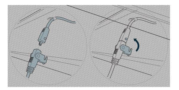
Locate the pre-installed power cord underneath the back of the converter's top tray. Join the power adapter cable to the pre-installed power cord, then secure the connection by latching the hook. Plug the converter into an outlet.
