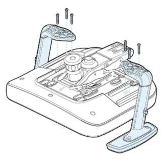
With the seat pan upside down, align the arm mounting holes with the holes on the seat pan. Noting the L and R marks on the seat pan and arms, ensure the chair arms are on the correct sides; the longer underside of the chair arm should be pointing toward the front of the seat pan (marked with an arrow). Bolting the arms on, using the six (6) M6 x 40mm screws and Allen key to secure them.
