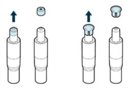
Remove the protective cap (could be orange or black) from the smaller end of the piston. Once the chair is assembled, the cap is no longer needed and can be discarded.
