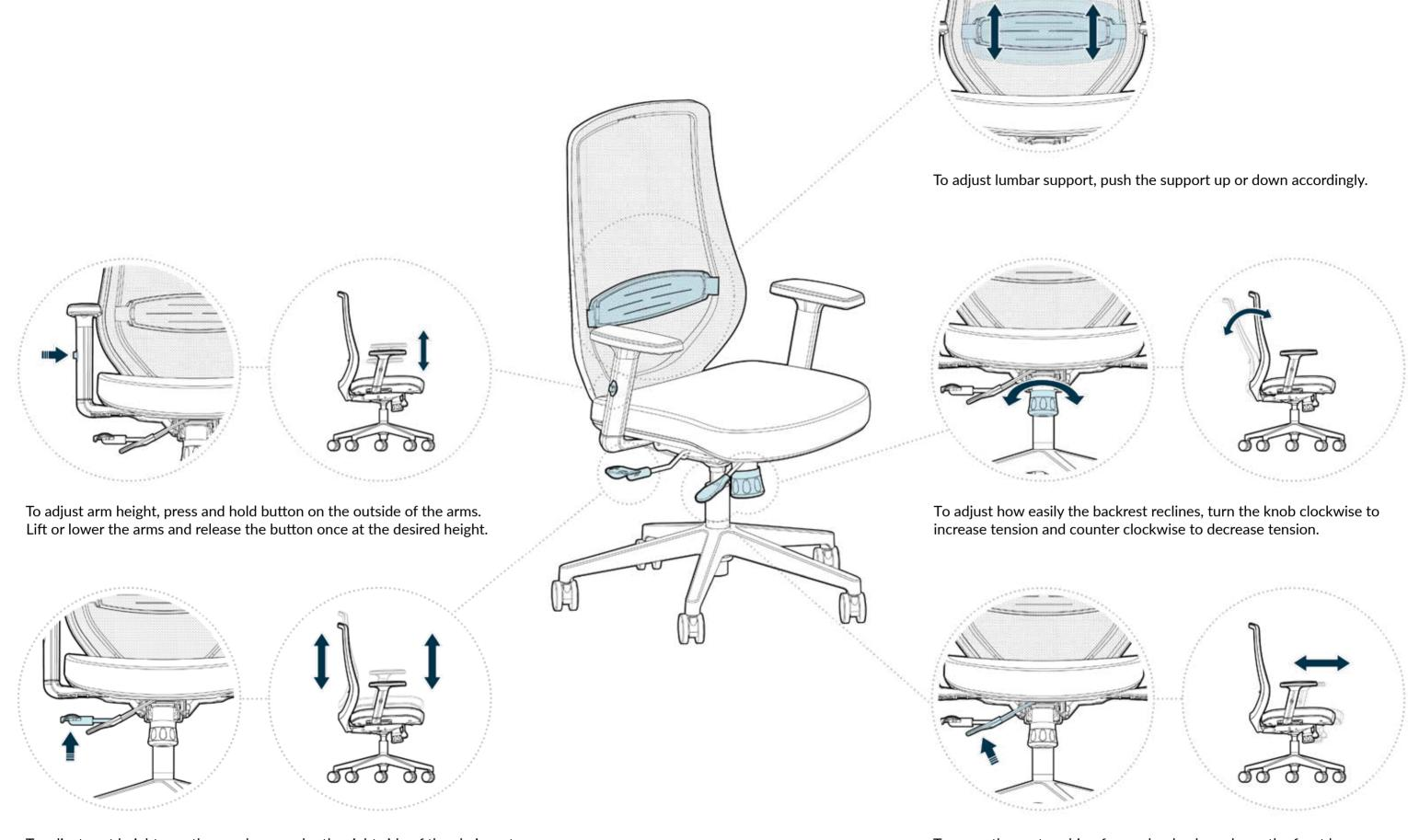
To adjust seat height, use the rear lever under the right side of the chair seat. This lever can also be pushed in to lock the backrest's angle or pulled out to allow the backrest to recline.
