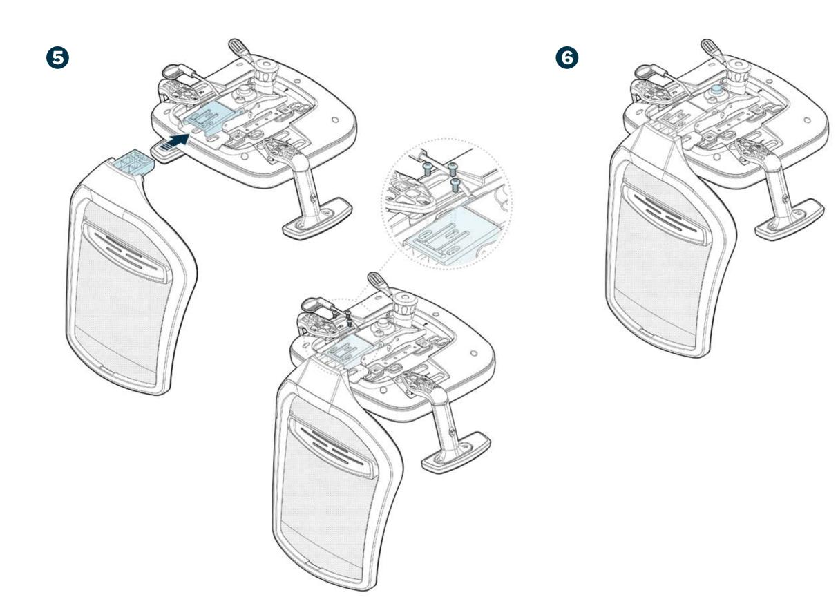
Slide the chair back onto the seat pan and align mounting holes. Use the three (3) M8 x 16mm screws and Allen key to secure the chair back.
